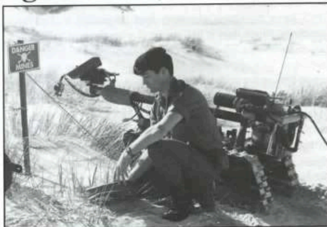
Robot mine clearance vehicle at work in the Falklands. Photo Harold Briley
